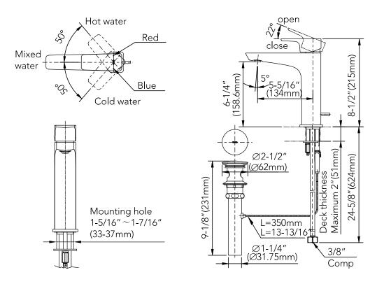
NOTE: The above dimensional unit is inch. The dimension in ( ) is reference mm.
