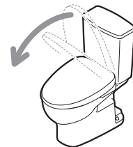
Toilet lid closes (About 90 seconds after standing up from the toilet seat.)
