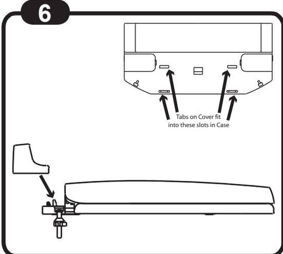
Install rear Hinge Cover by fitting the tabs on the rear Cover into the slits on the Hinge Case.
