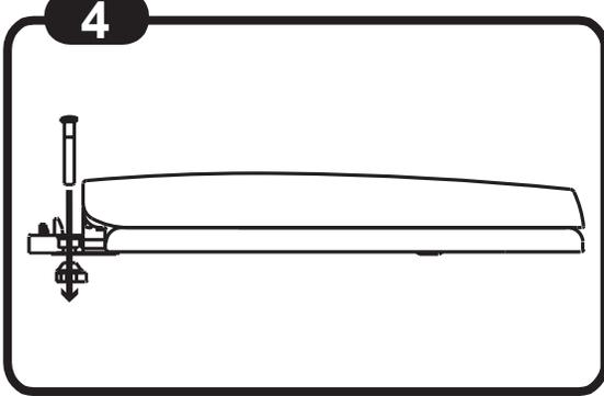
Insert Plastic Bolt (B) and tighten Plastic Nut (C) on underside of toilet.
