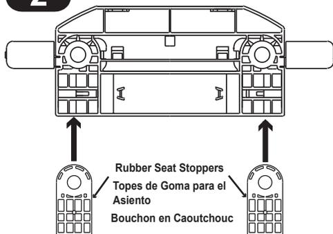
Add anti-skid, Rubber Seat Stoppers (A) to the corresponding grooves on the bottom of the Hinge Case. Make sure the Rubber Seat Stoppers lie flat against the Hinge Case.
