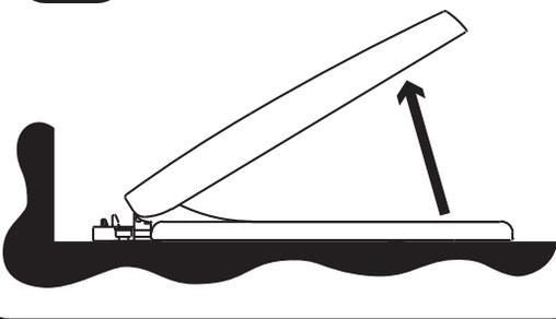
Flatten the Hinge Case against the toilet by holding the seat down and raising the lid. Hold the Hinge Case against the toilet and lower the lid.
